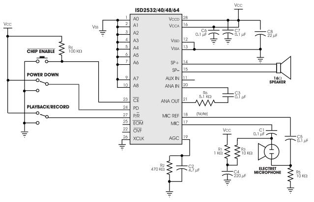
Figure 4: ISD2500 Application Example—Design Schematic
