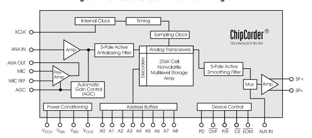
Figure i: ISD2532/40/48/64 Device Block Diagram
