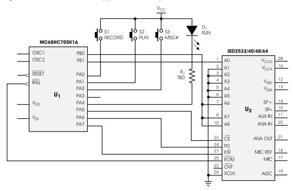
Figure 5: ISD2532/40/48/64 Application Example—Microcontroller/ISD2500 Interface
