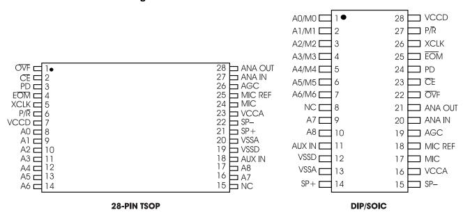
Figure 1: ISD2532/40/48/64 Device Pinouts
