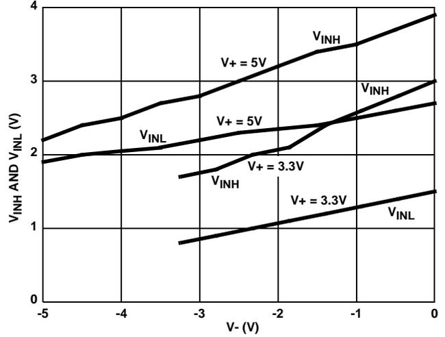
FIGURE 14. DIGITAL SWITCHING POINT vs NEGATIVE SUPPLY VOLTAGE
