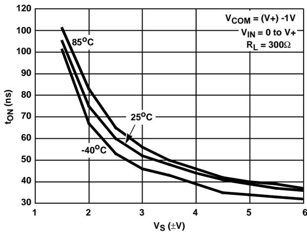
FIGURE 11. TURN - ON TIME vs SUPPLY VOLTAGE
