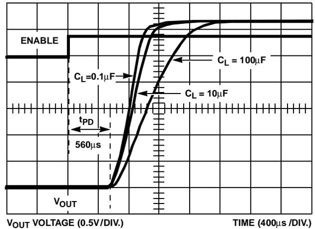
FIGURE 3. V<sub>OUT</sub> SOFT START vs C<sub>L</sub> and PROP DELAY, R<sub>I</sub> = 8Ω
