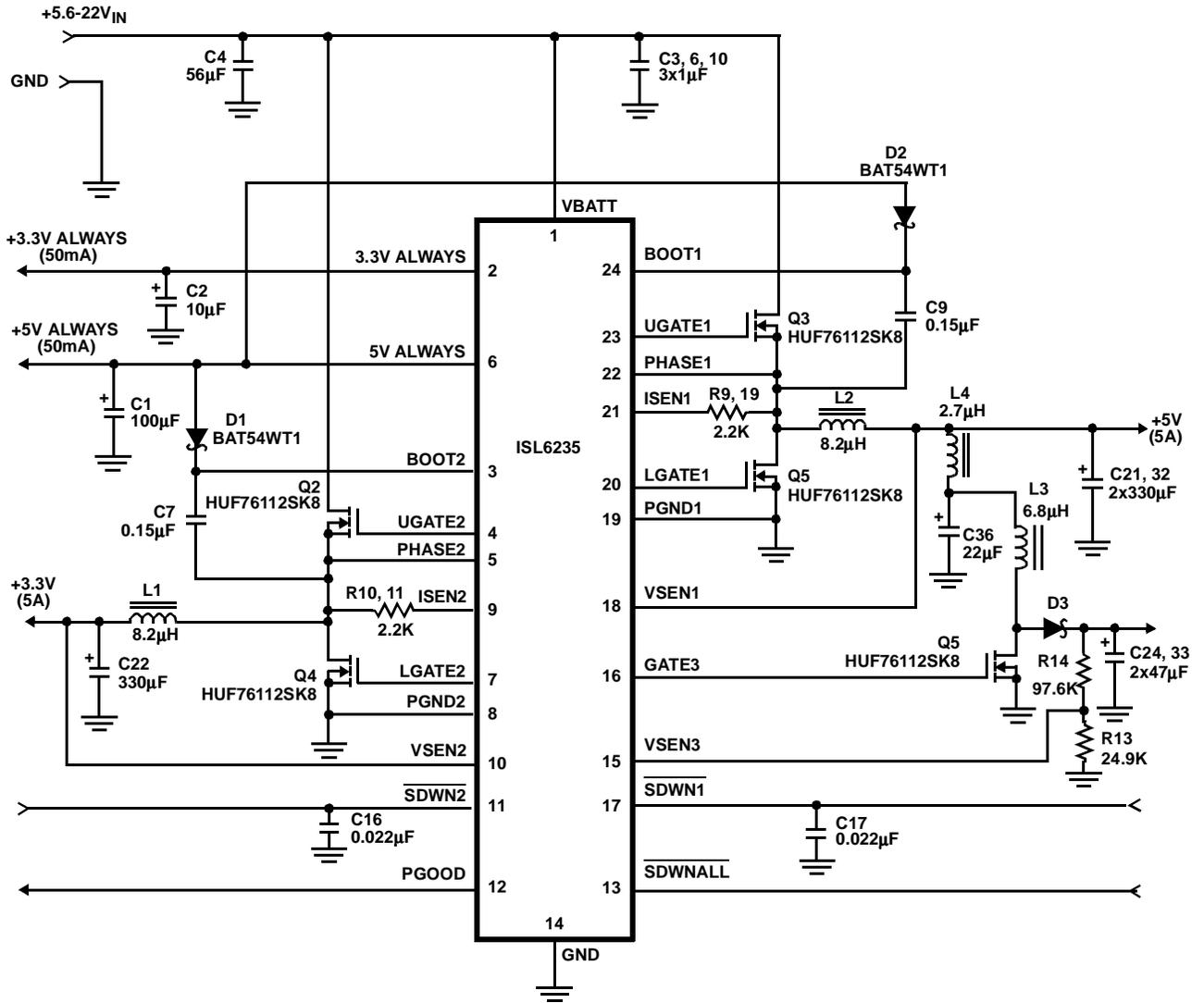
FIGURE 6. APPLICATIONS CIRCUIT
