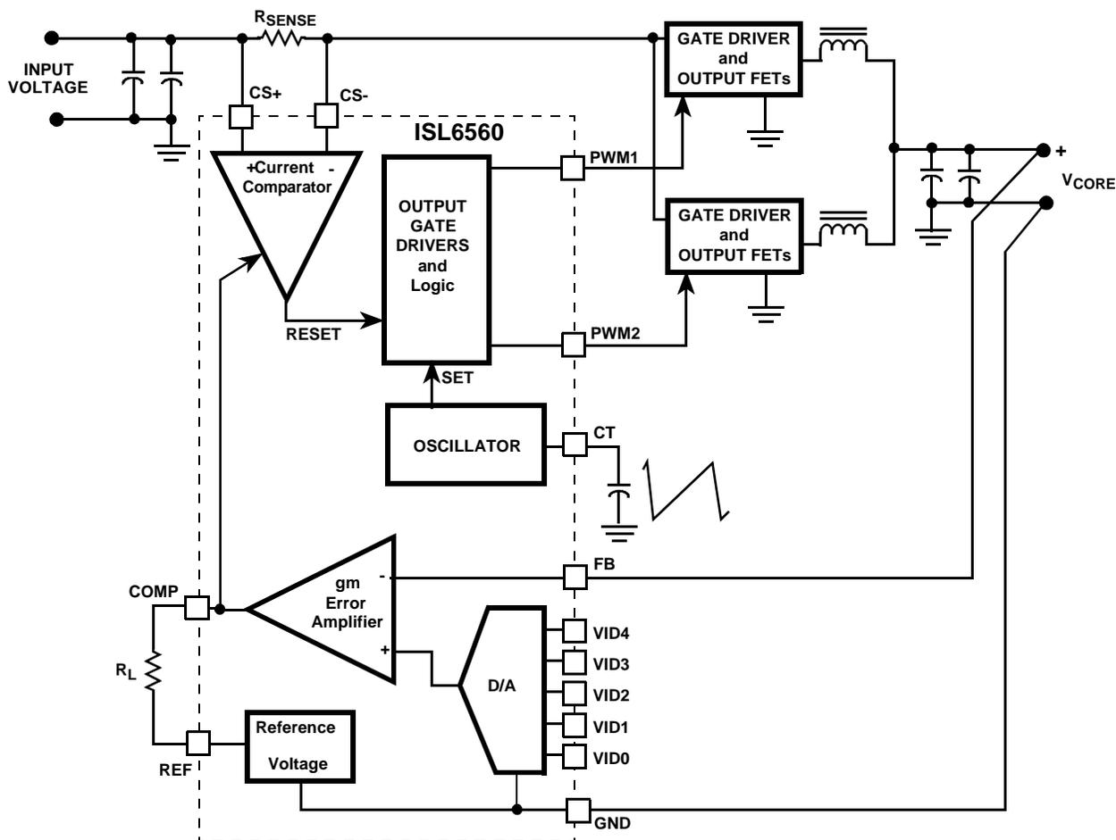
FIGURE 1. FUNCTIONAL SYSTEM BLOCK DIAGRAM SHOWING MAJOR COMPONENTS
