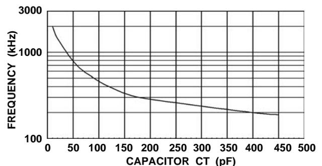
FIGURE 3. OSCILLATOR FREQUENCY vs. TIMING CAPACITOR
