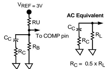
FIGURE 9. COMPENSATION CIRCUIT
