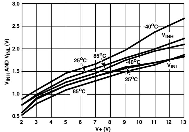
FIGURE 10. DIGITAL SWITCHING POINT vs SUPPLY VOLTAGE
