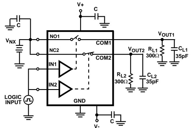
$C_L$  includes fixture and stray capacitance.
