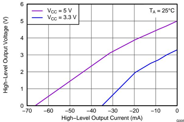
Figure 11. High-Level Output Voltage vs High-Level Output Current
