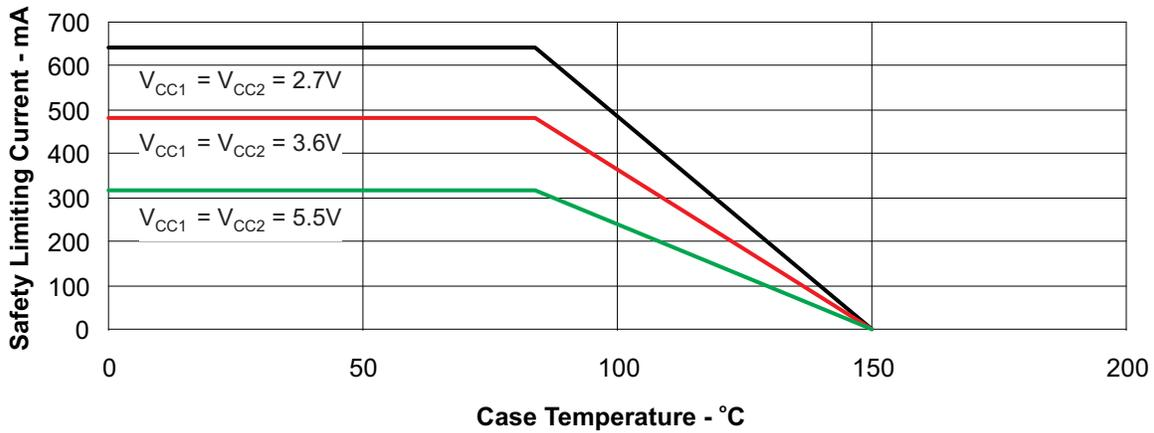
Figure 5. DW-16  $\theta_{JC}$  Thermal Derating Curve per IEC 60747-5-2
