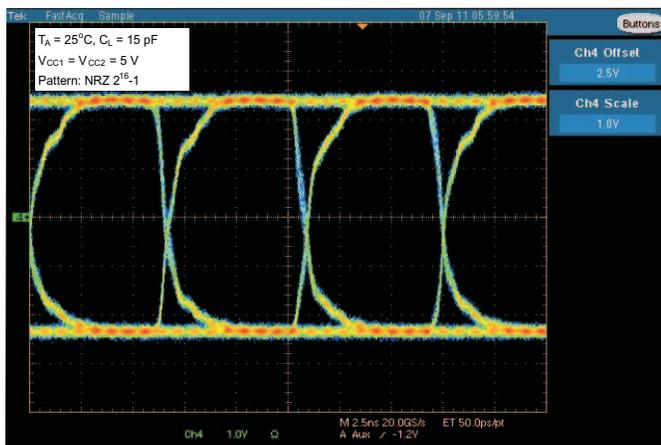
Figure 16. Typical Eye Diagram at 150 Mbps, 5 V Operation
