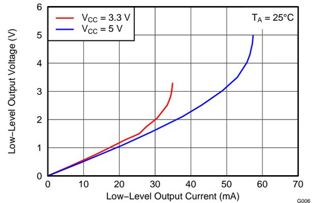
Figure 12. Low-Level Output Voltage vs Low-Level Output Current
