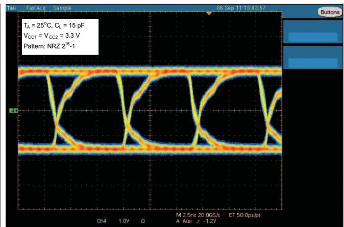
Figure 17. Typical Eye Diagram at 150 Mbps, 3.3 V Operation
