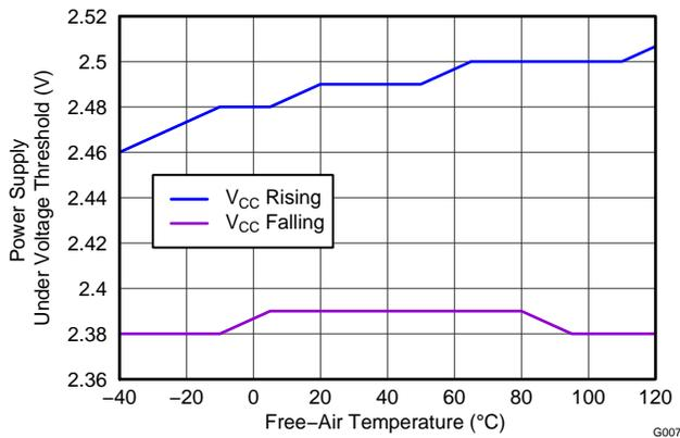
Figure 13. V<sub>CC</sub> Undervoltage Threshold vs Free Air Temperature
