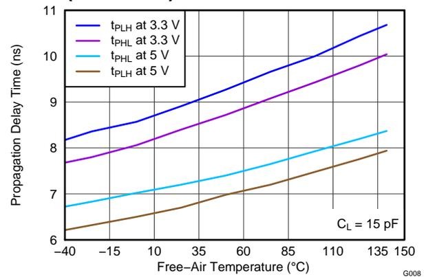
Figure 14. Propagation Delay Time vs Free Air Temperature
