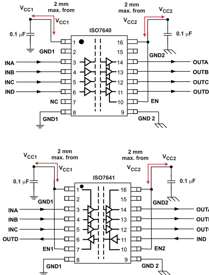
Figure 6. Typical ISO7640FM and ISO7641FM Application Circuit
