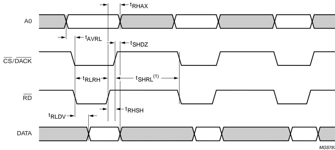
(1) For  $t_{SHRL}$ , both  $\overline{CS}$  and  $\overline{RD}$  must be de-asserted.
