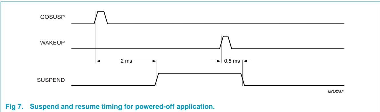
**Fig 7. Suspend and resume timing for powered-off application.**
