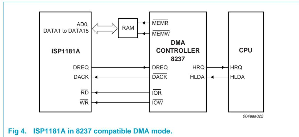
Fig 4. ISP1181A in 8237 compatible DMA mode.
