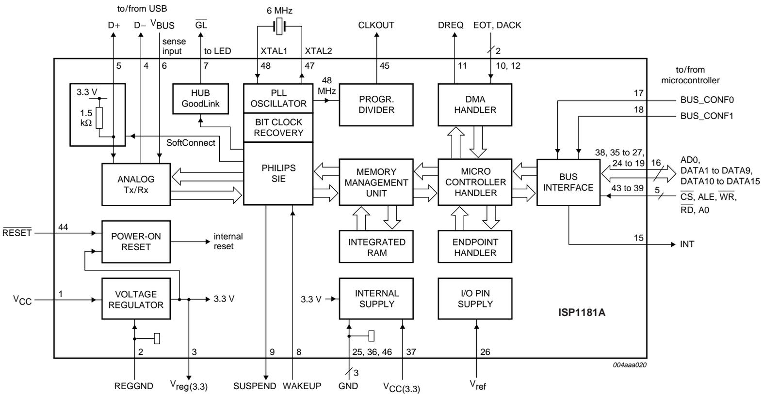
Fig 1. Block diagram.
