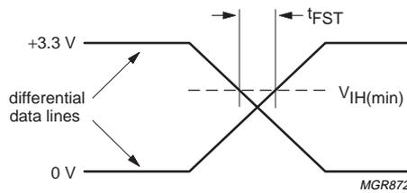
**Fig 18. Receiver SE0 width tolerance.**
