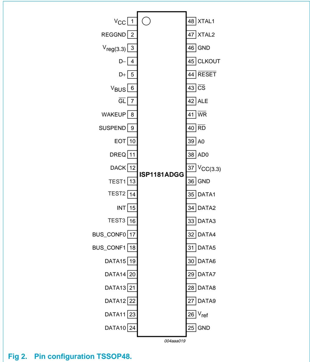
Fig 2. Pin configuration TSSOP48.
