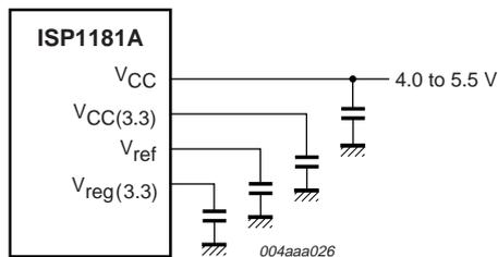
Fig 10. ISP1181A with a 4.0 to 5.5 V supply.
