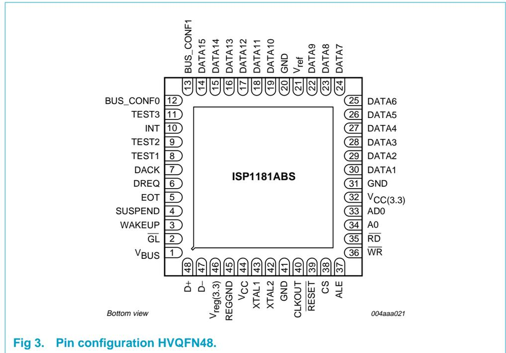
Fig 3. Pin configuration HVQFN48.
