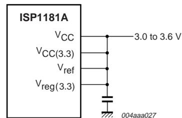
Fig 11. ISP1181A with a 3.0 to 3.6 V supply.
