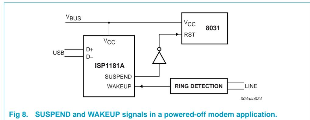
Fig 8. SUSPEND and WAKEUP signals in a powered-off modem application.
