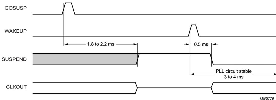
If enabled, the 100 ± 50% kHz LazyClock frequency will be output on pin CLKOUT during 'suspend' state.
