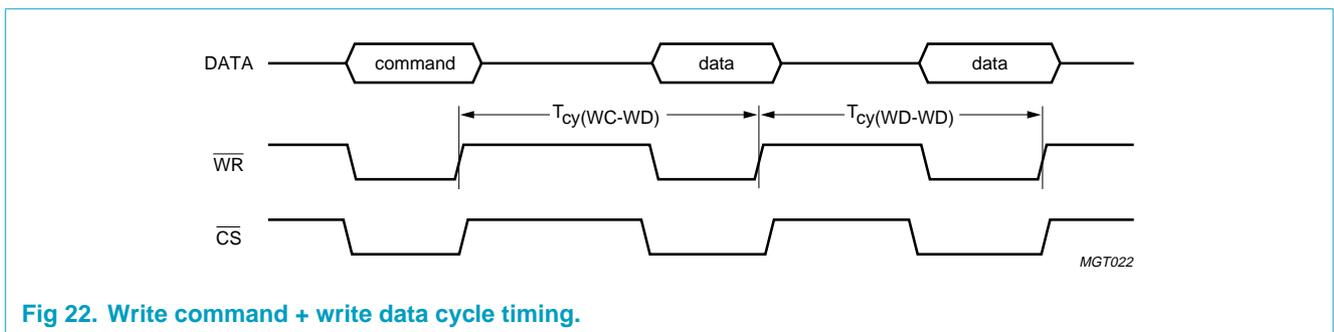
Fig 22. Write command + write data cycle timing.
