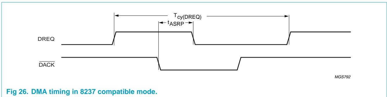
Fig 26. DMA timing in 8237 compatible mode.
