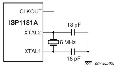
Fig 12. Typical oscillator circuit.
