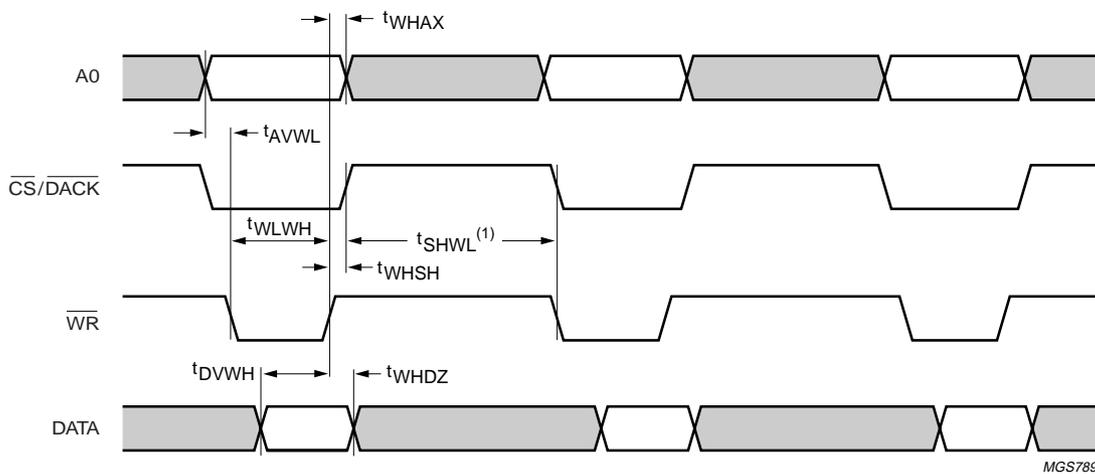
(1) For  $t_{SHWL}$ , both  $\overline{CS}$  and  $\overline{WR}$  must be de-asserted.
