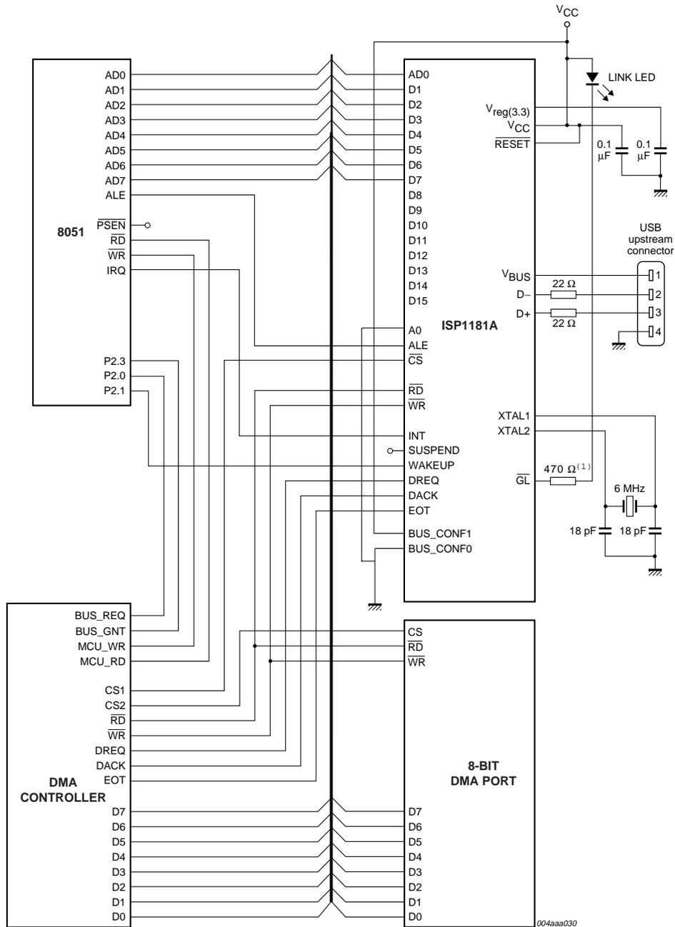
(1) Use of a 470 Ω resistor assumes that V<sub>CC</sub> is 5.0 V.
