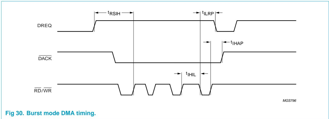
Fig 30. Burst mode DMA timing.
