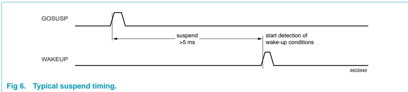
**Fig 6. Typical suspend timing.**
