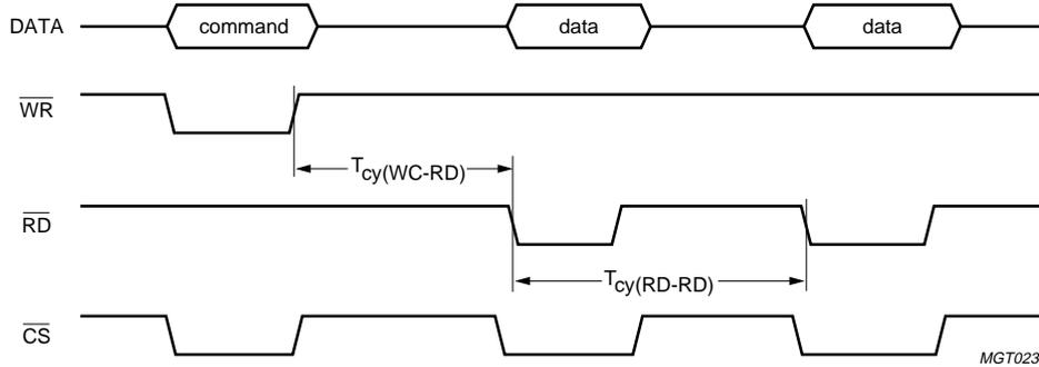
Fig 24. Write command + read data cycle timing.
