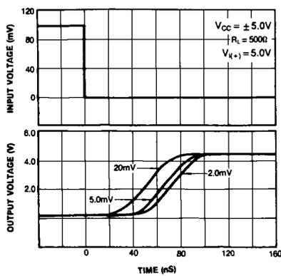
Fig. 6 INPUT CHARACTERISTICS
