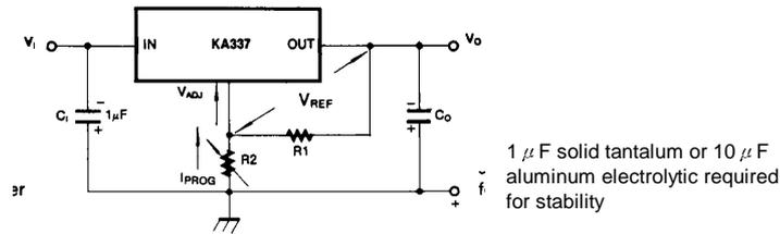
1  $\mu$  F solid tantalum or 10  $\mu$  F aluminum electrolytic required for stability
