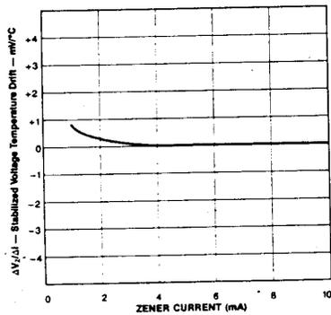
Figure 9. Stabilized Voltage Temperature Drift vs. Zener Current
