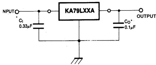
A common ground is required between the Input and the output voltages. The input voltage must remain typically 2.0V above the output voltage even during the low point on the input ripple voltage.
