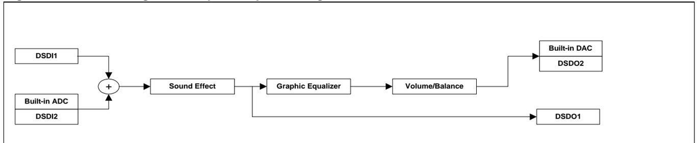
For this configuration, one should set Mixing to be turned on and Bypass On-Chip Function to be turned off. Input signals from different sources can be mixed with controllable gains. After mixed, the flow is identical to Configuration 1 and 3. To obtain Configuration 4, one can send host commands from microcontroller in the order of the commands listed in Table 16.
