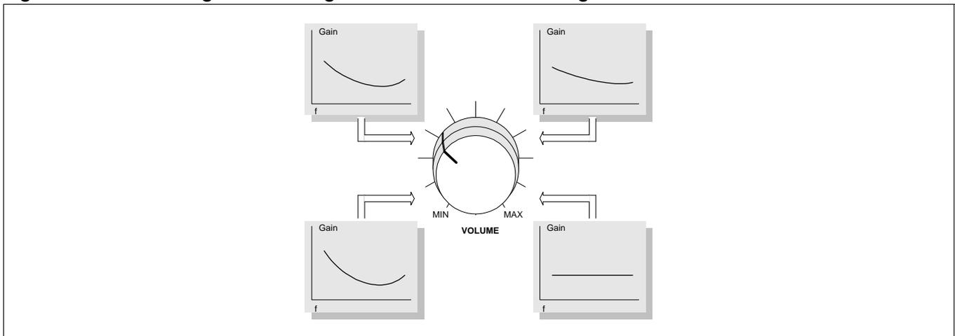
**Figure 20. Loudness compensated level with respect to volume level**
