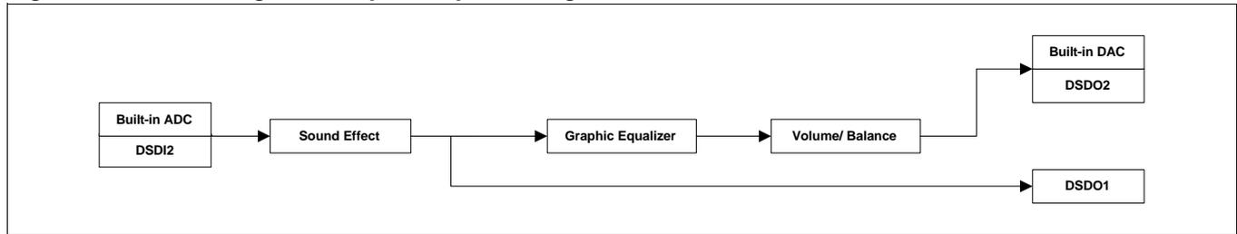
This configuration is exactly same as Configuration 1 except for input source. For this configuration, one should set Mixing and Bypass On-Chip Function to be turned off while the built-in ADC or DSDI2 is enabled. To obtain Configuration 3, one can send host commands from microcontroller in the order of the commands listed in Table 15.
