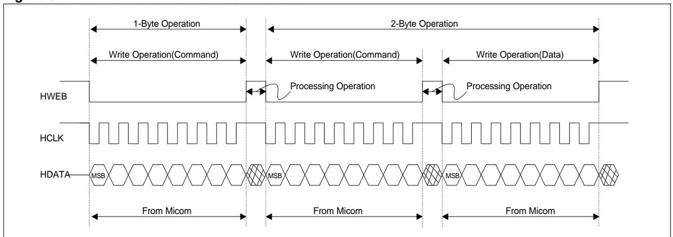
**Figure 7. Data Format in Normal Host Interface-Spectrum Request**
