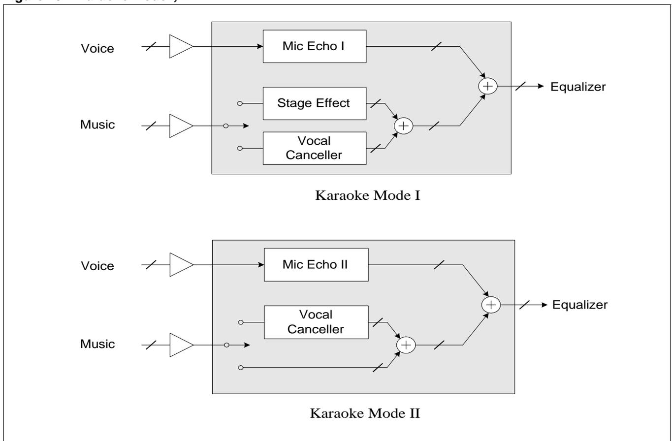
In Mic echo filter 1, the delay gains remain large and they are shortly decayed as time goes by. Thus, one can feel plenty of echo while there is little aliasing between echos and original sound. The Mic echo filter 2 has a similar structure to that of Hall mode. The effect is not stronger than that of Mic echo filter 1, but it produces a widely spread echo which is very impressive.
