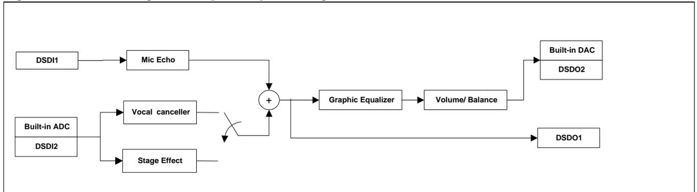
This configuration is also for Karaoke mode I as shown in Configuration 5. The difference between them is that sources for mic-echo and stage effect mode are exchanged. To obtain this configuration, one should set Input Source Selection in Karaoke I to be inverted and other switches (Mixing, Bypass On-Chip Function) to be turned off. To obtain Configuration 6, one can send host commands from microcontroller in the order of the commands listed in Table 18.
