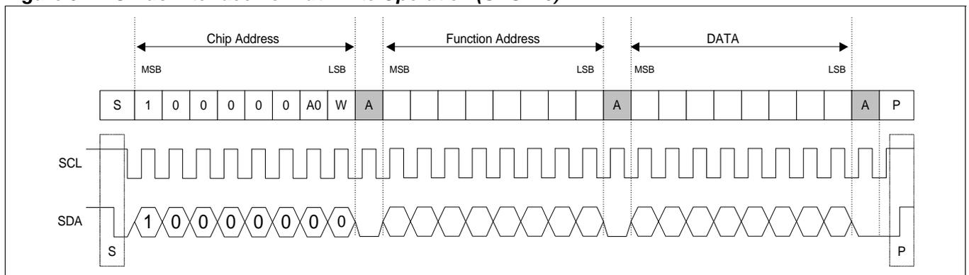
Figure 10. I<sup>2</sup>C Bus Interface Format-Read Operation (SAS = 0)
