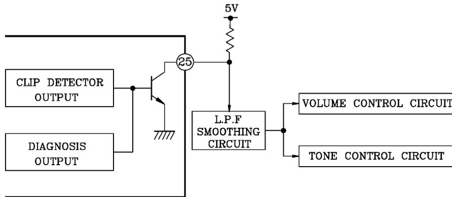
PIN <sup>25</sup> : Open Collector Output (Active Low)
