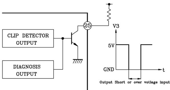
PIN <sup>25</sup> : Open Collector Output (Active Low)
