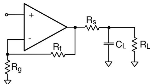
**Figure 4: Typical Topology for driving a capacitive load**
