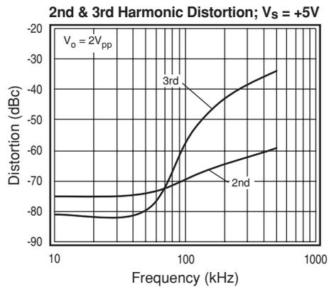
**KM4212 Performance Characteristics** ( $V_s = +5V$ ,  $G = 2$ ,  $R_L = 10k\Omega$  to  $V_s/2$ ,  $R_f = 10k\Omega$ ; unless noted)
