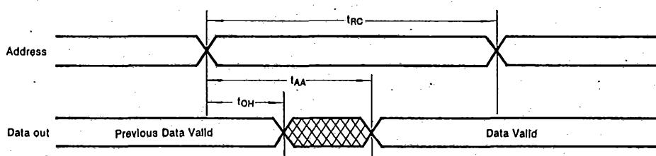
TIMING WAVEFORM OF READ CYCLE NO. 2 ( $WE = V_{IH}$ )
