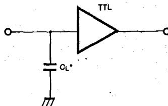
\* Including Scope and Jig Capacitance
