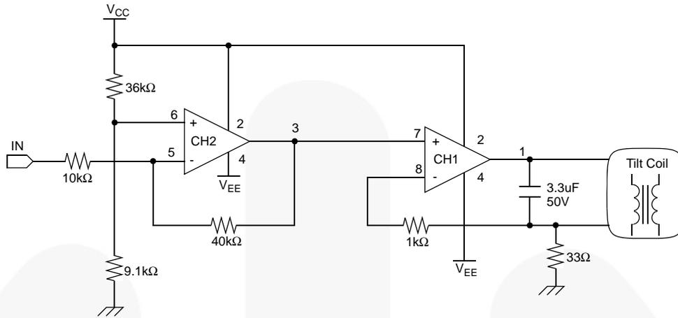
Figure 7. Tilt Coil, Current-Control Circuit in Monitor
