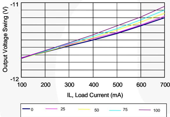
Figure 4. Output Voltage Swing vs. Load Current
