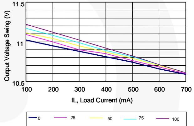
Figure 5. Output Voltage Swing vs. Load Current
