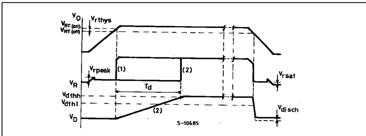
put instantaneously goes down (LOW status) inhibiting the microprocessor. The typical power on-off hysteresis is 50mV.
