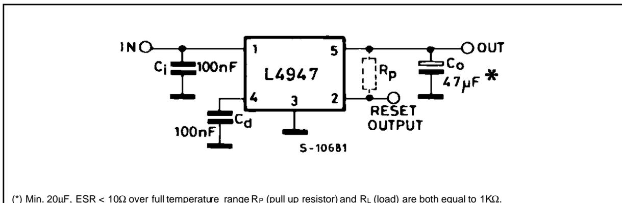
**ELECTRICAL CHARACTERISTICS** (refer to the test circuit,  $V_i = 14.4\text{V}$ ,  $C_o = 47\mu\text{F}$ ,  $\text{ESR} < 10\Omega$ ,  $R_p = 1\text{K}\Omega$ ,  $R_L = 1\text{K}\Omega$ ,  $-40^\circ\text{C} \leq T_J \leq 125^\circ\text{C}$ , unless otherwise specified)
