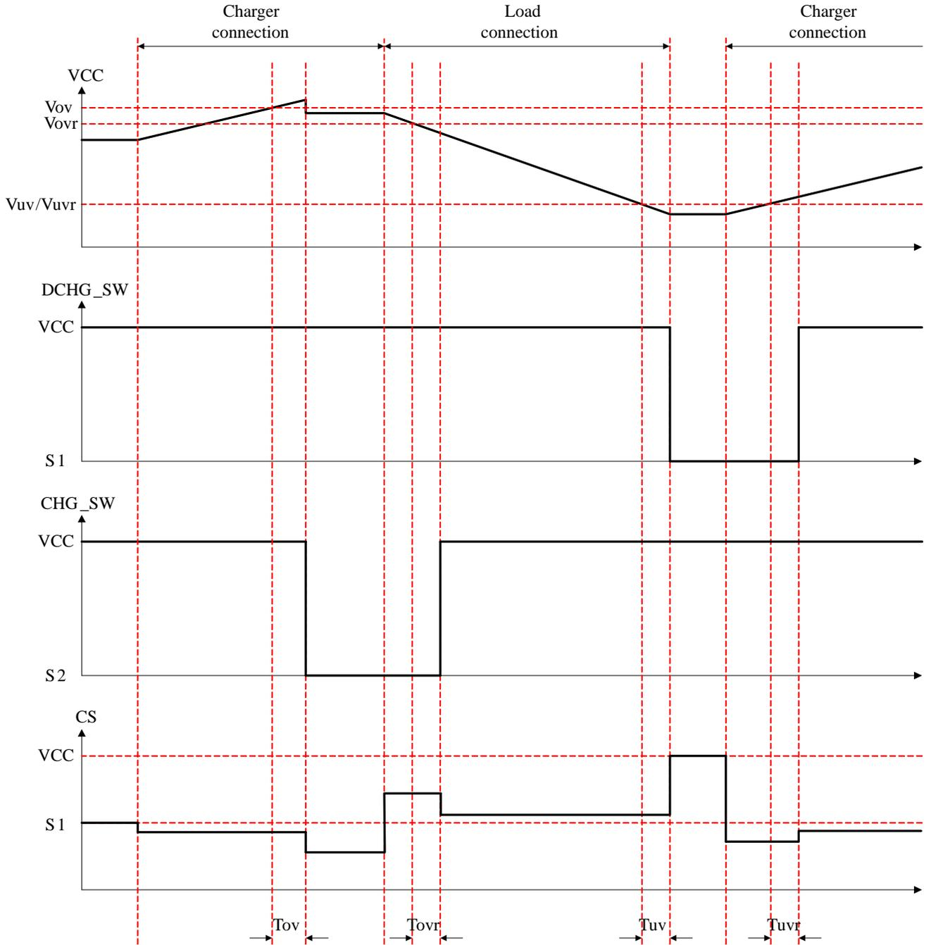
Figure 6. Over-charged detection/release, Over-discharge detection/release (Connect charger)
