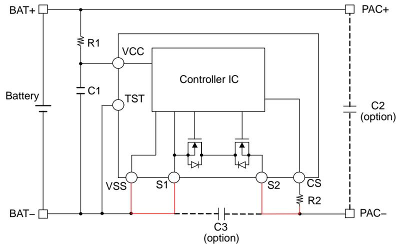
Figure 2. Board Schematic
