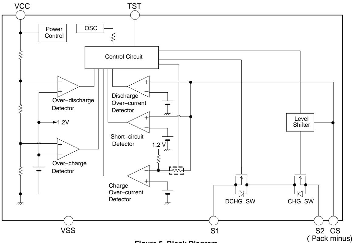
**Figure 5. Block Diagram**
