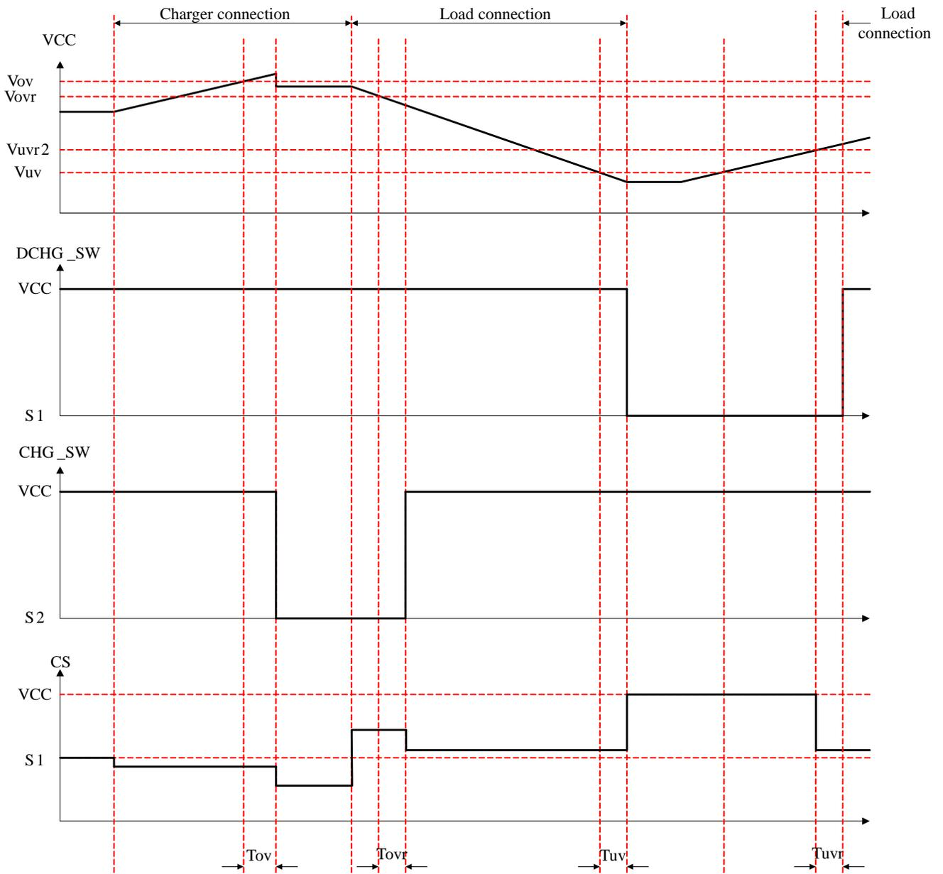
Figure 7. Over-charge detection/release, Over-discharged detection/release (Non-connect charger)
