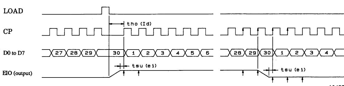
Note: 2. If this IC is used with a 4-bit width data input, the number of data clocks between one LOAD and the next LOAD must be doubled.
