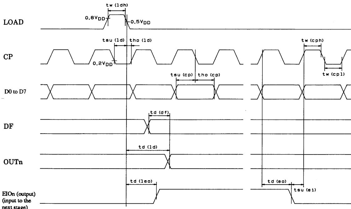
Note: 1. Since this IC detects the EIO inputs on the rising edge of the CP signal, the EIO inputs must be set up before the first data is input. As a result, a  $t_{ho}(ld)$  clock stop period is required directly after the rise of the LOAD signal if the clock frequency is relatively high.
