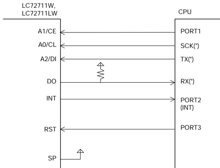
\* SCK, TX, and RX are the CPU serial interface channel. Normally, I/O port pins may be used for these lines.
