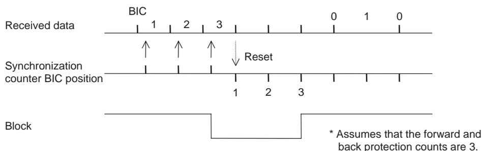
Figure 1 Block Synchronization Protection Operation (Forward → Back → Forward)
