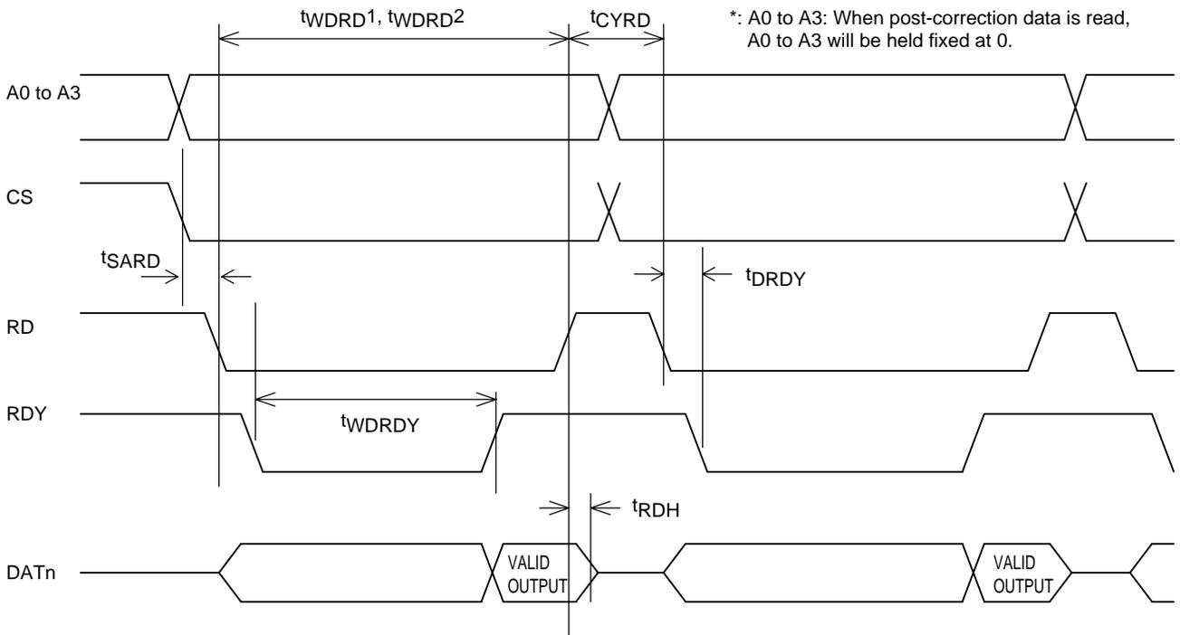
• Post-Correction Data Read Timing (DMA)
