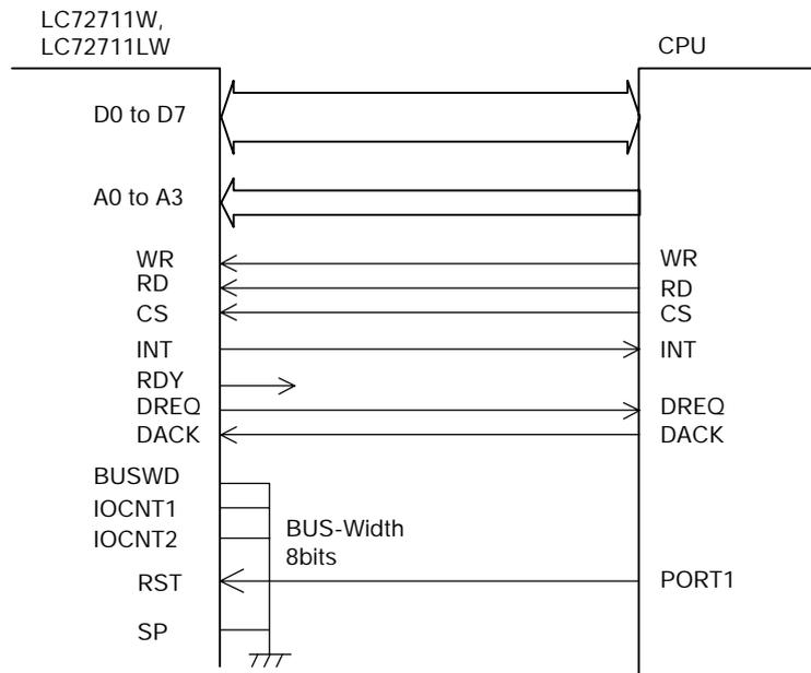
CPU DMA mode setting example
