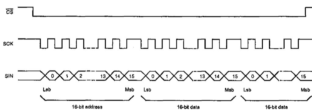
Only the lower eight bits of the address word are significant. Only the lower eight bits of data words at addresses 000H to 0AFH, the lower 11 bits of data
