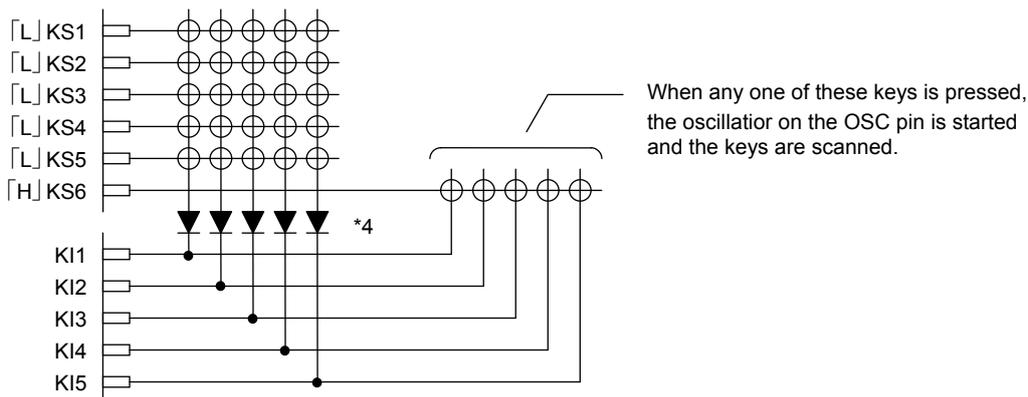
Note: \*4. These diodes are required to reliably recognize multiple key presses on the KS6 line when sleep mode state with only KS6 high, as in the above example. That is, these diodes prevent incorrect operations due to sneak currents in the KS6 key scan output signal when keys on the KS1 to KS5 lines are pressed at the same time.
