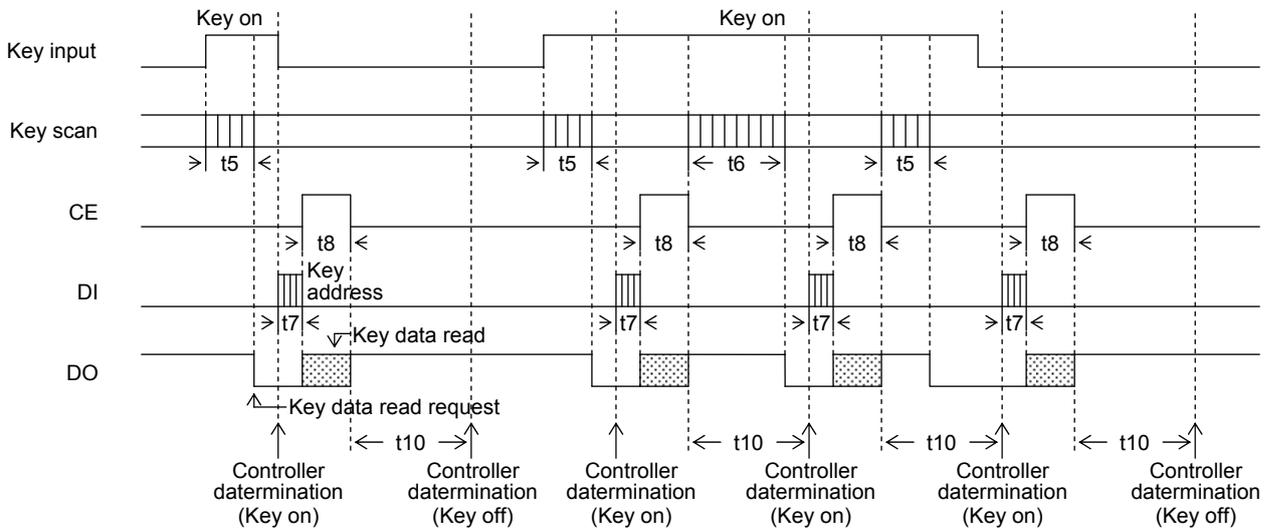
t5 ..... Key scan execution time when the key data agreed for two key scans. (615T(s))
