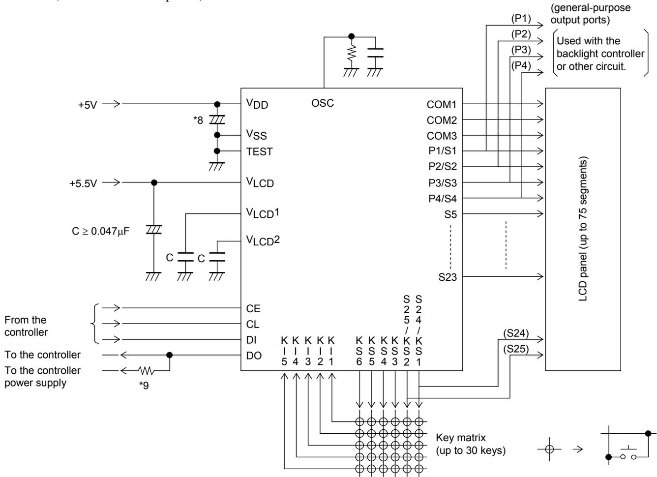
Note: \*8. Add a capacitor to the logic block power supply line so that the logic block power supply voltage  $V_{DD}$  rise time when power is applied and the logic block power supply voltage  $V_{DD}$  fall time when power drops are both at least 1 ms, as the LC75863W is reset by the  $V_{DET}$ .
