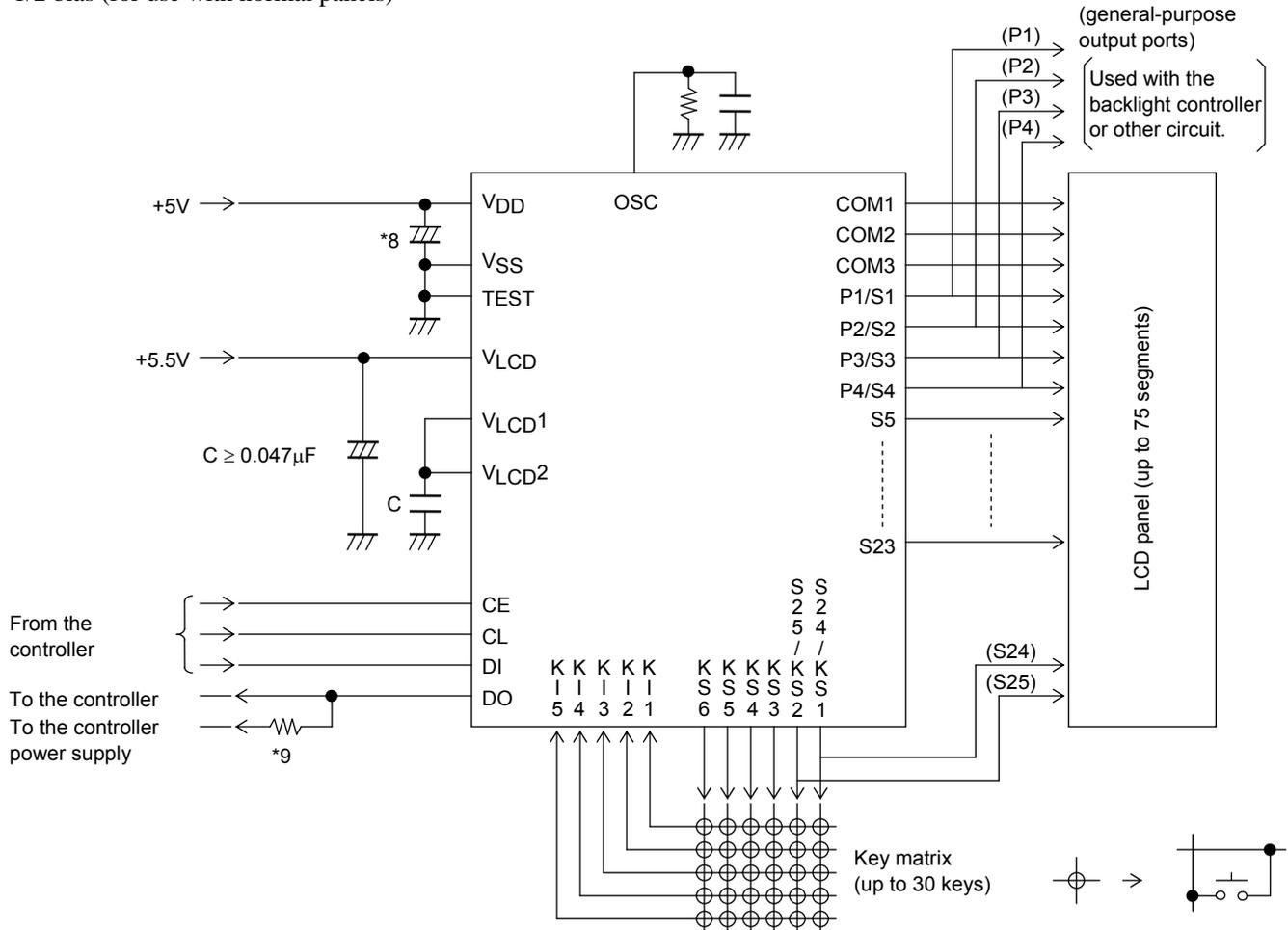
Note: \*8. Add a capacitor to the logic block power supply line so that the logic block power supply voltage  $V_{DD}$  rise time when power is applied and the logic block power supply voltage  $V_{DD}$  fall time when power drops are both at least 1 ms, as the LC75863W is reset by the  $V_{DET}$ .
