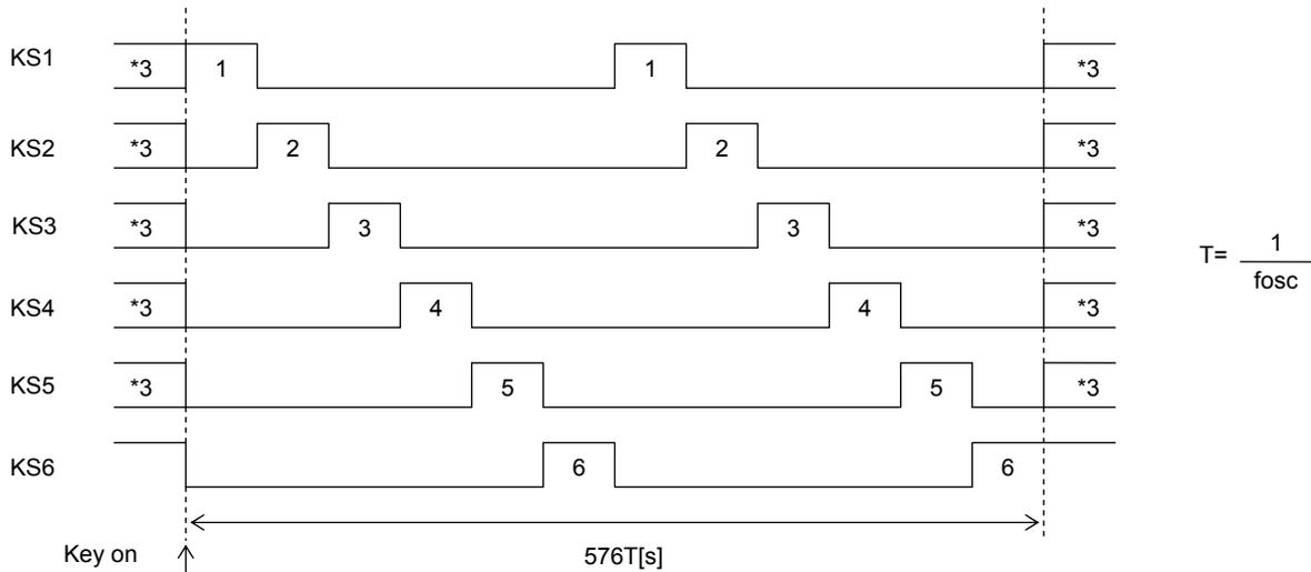
Note: \*3. In sleep mode the high/low state of these pins is determined by the S0 and S1 bits in the control data. Key scan output signals are not output from pins that are set low.
