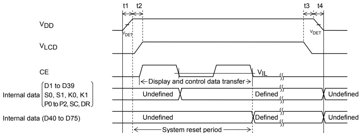
Note:  $t_1 \geq 1$  [ms] (Logic block power supply voltage  $V_{DD}$  rise time)
