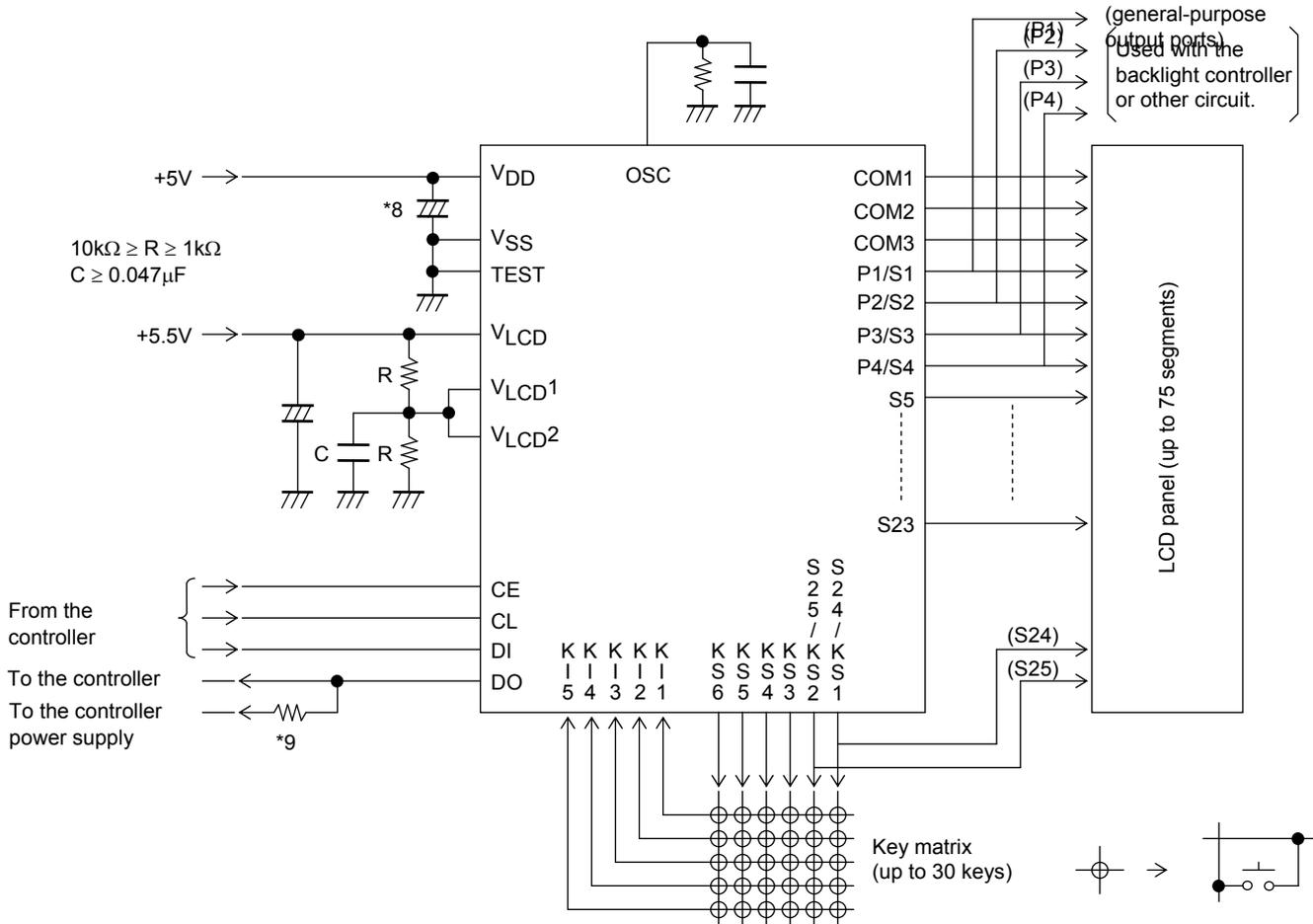
Note: \*8. Add a capacitor to the logic block power supply line so that the logic block power supply voltage V<sub>DD</sub> rise time when power is applied and the logic block power supply voltage V<sub>DD</sub> fall time when power drops are both at least 1 ms, as the LC75863W is reset by the V<sub>DET</sub>.
