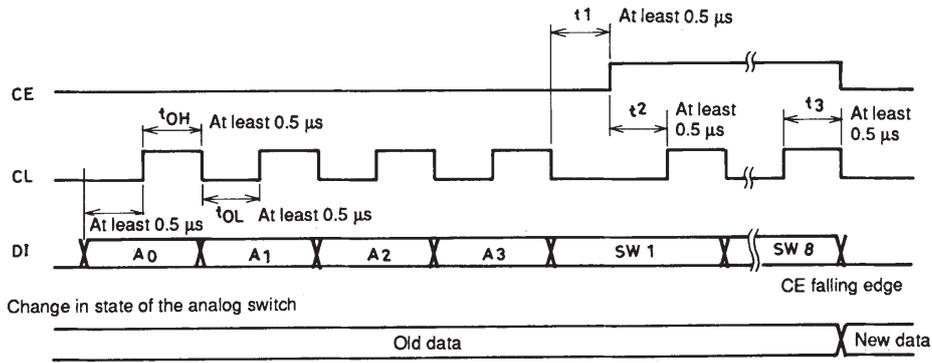
Data is read in on the rising edge of CL and latched on the falling edge of CE.
