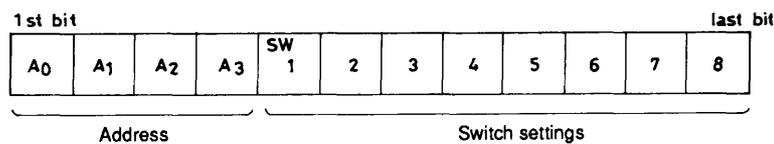
Bits correspond to the L1 to L8 and R1 to R8 analog switches, and a value of one turns the corresponding switch on, and a value of zero turns it off.
