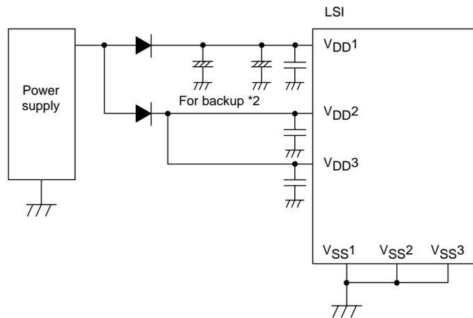
\*2: The internal memory is sustained by  $V_{DD1}$ . If none of  $V_{DD2}$  and  $V_{DD3}$  are backed up, the high level output at the ports are unstable in the HOLD backup mode, allowing through current to flow into the input buffer and thus shortening the backup time.
