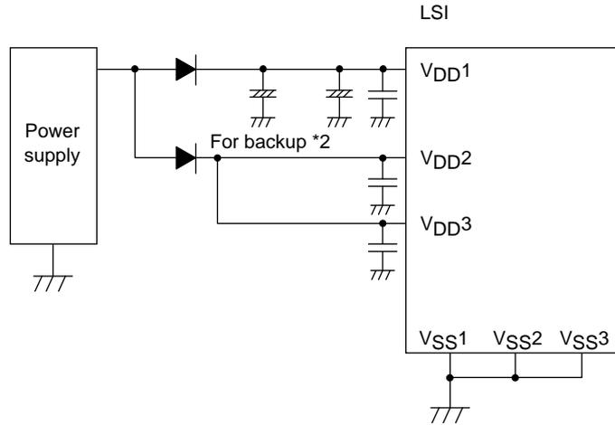
\*2 The internal memory is sustained by VDD1. If none of VDD2 and VDD3 are backed up, the high level output at the ports are unstable in the HOLD backup mode, allowing through current to flow into the input buffer and thus shortening the backup time. Make sure that the port outputs are held at the low level in the HOLD backup mode.
