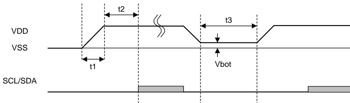
Figure 8.1 V<sub>DD</sub> supply timing
