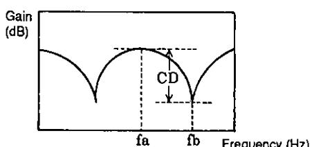
5. Measure the C-OUT output with a 200 mVp-p sine wave signal input to C-IN1 and C-IN2 and with 500 mVp-p sine wave signal input and calculate the difference in the gains.
