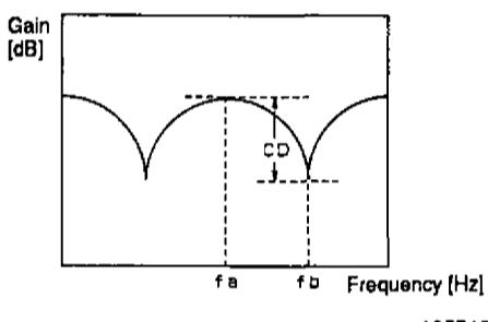
5. Measure the C-OUT output when 200-mVp-p sine wave signals are input to C-IN1 and C-IN2 and when 500-mVp-p sine wave signals are input and calculate the gain difference.
