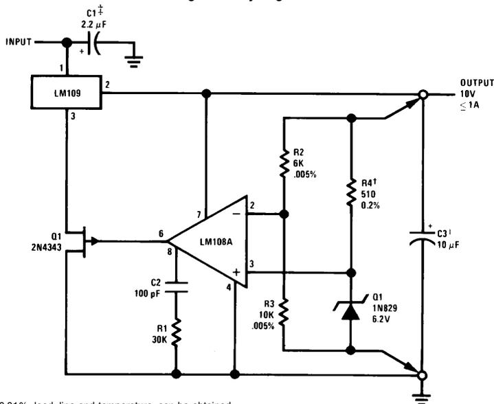
\*Regulation better than 0.01%, load, line and temperature, can be obtained.
