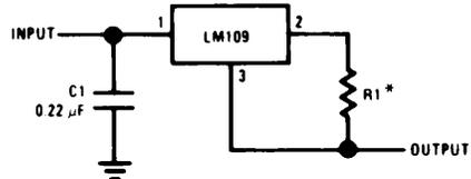
\*Determines output current. If wirewound resistor is used, bypass with 0.1 μF.
