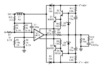
Discrete transistors can be used to increase output drive to  $\pm 70V$  at  $\pm 10A$  as shown above. With proper thermal design, the IC will provide safe-area protection for the external transistors. Voltage gain is about thirty.
