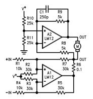
Although op amps are usually operated from dual supplies, single-supply operation is practical. This bridge amplifier supplies bi-directional current drive to a servo motor while operating from a single positive supply. The output is easily converted to voltage drive by shorting  $R_6$  and connecting  $R_7$  to the output of  $A_2$ , rather than  $A_1$ .
