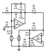
This motor/tachometer servo gives an output speed proportional to input voltage. A low-level op amp is used for frequency shaping while the power op amp provides current drive to the motor. Current drive eliminates loop phase shift due to motor inductance and makes high-performance servos easier to stabilize.
