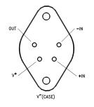
4-pin glass epoxy TO-3 socket is available from AUGAT INC. Part number 8112-AG7
