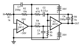
This circuit shows how two amplifiers can be cascaded to double output swing. The advantage over the bridge is that the output can be increased with any number of stages, although separate supplies are required for each.
