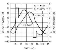
Should the power ratings of the LM12 be exceeded, dynamic safe-area protection is activated. Waveforms with this power limiting are shown for the LM12 driving  $\pm 26V$  at 30 Hz into 3 $\Omega$  in series with 24 mH ( $\theta$  = 45°). With an inductive load, the output clamps to the supplies in power limit, as above. With resistive loads, the output voltage drops in limit. Behavior with more complex RCL loads is between these extremes.
