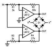
The voltage swing delivered to the load can be doubled by using the bridge connection shown here. Output clamping to the supplies can be provided by using a bridge-rectifier assembly.
