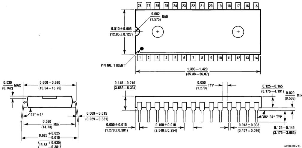
**28-Lead (0.600" Wide) Molded Dual-In-Line Package
