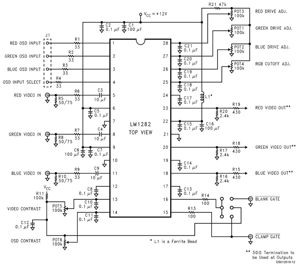
**FIGURE 7. LM1282 OSD Video Preamp Demonstration Board Schematic**
