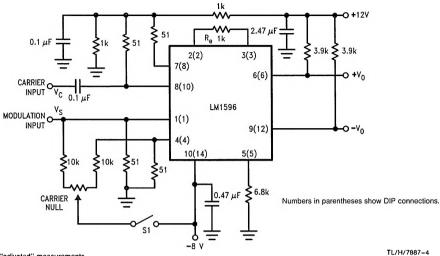
Note: S<sub>1</sub> is closed for "adjusted" measurements.
