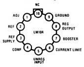
Note: Pin 5 connected to case.
