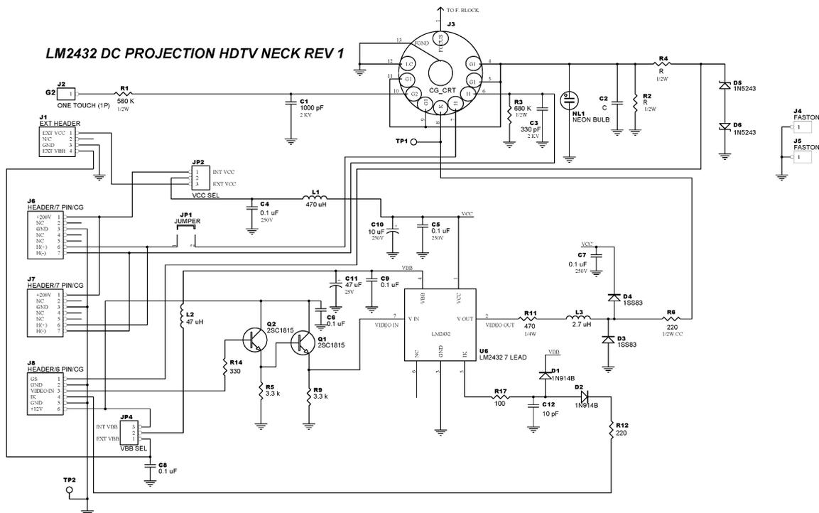
Figure 16. LM2432 Demonstration Board Schematic
