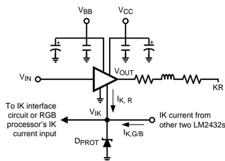
Figure 15. Simplified IK Interface for Current Feedback Systems
