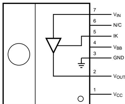
**Note:** Tab is at GND. Pin 6 is not connected (N/C) internally.
