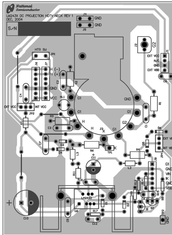
Figure 17. LM2432 Demonstration Board Layout
