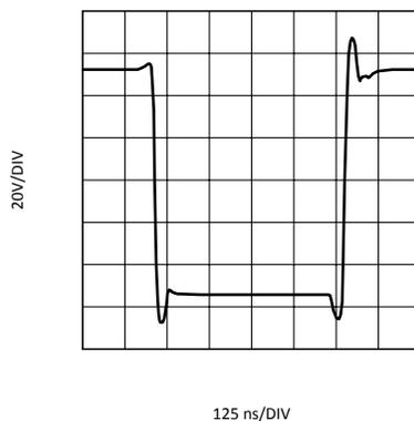
Figure 12. Cathode Pulse Response
