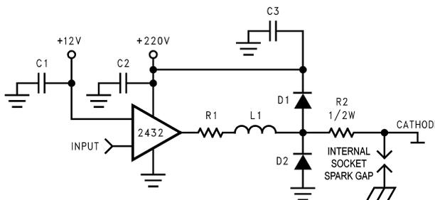
Figure 13. Recommended Application Circuit
