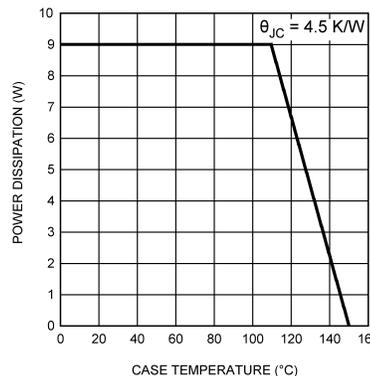
Figure 11. Power Derating Curve
