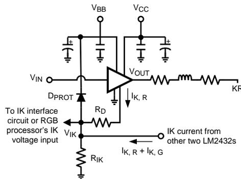
Figure 14. Simplified IK Interface for Voltage Feedback Systems
