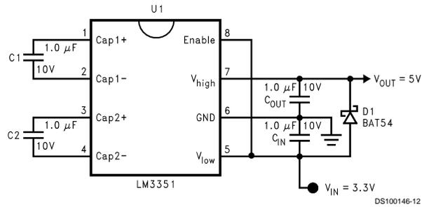
FIGURE 1. Step-Up Converter
