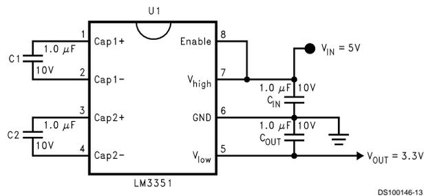
FIGURE 2. Step-Down Converter
