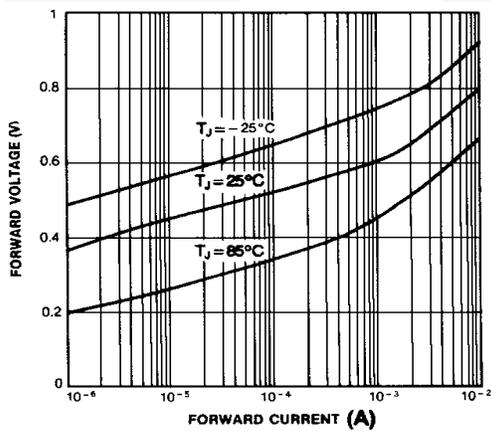
Figure 5. Forward Characteristics
