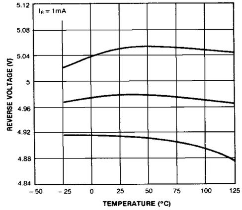
Figure 4. Temperature Drift
