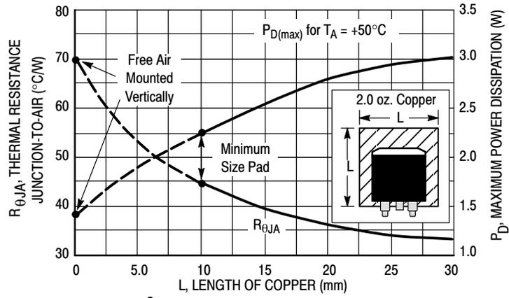
**Figure 19. D<sup>2</sup>PAK Thermal Resistance and Maximum Power Dissipation versus P.C.B. Copper Length**
