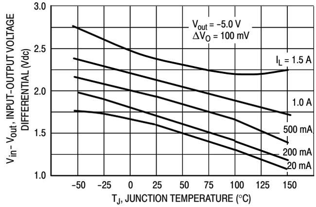
Figure 8. Dropout Voltage
