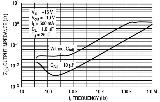
Figure 14. Output Impedance
