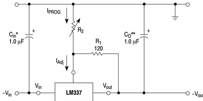
\*C<sub>in</sub> is required if regulator is located more than 4 inches from power supply filter. A 1.0 μF solid tantalum or 10 μF aluminum electrolytic is recommended.
