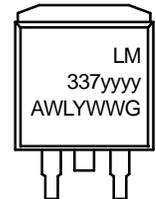
Heatsink surface (shown as terminal 4 in case outline drawing) is connected to Pin 2.
