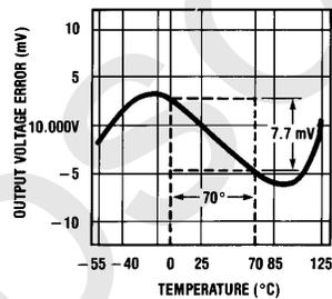
Typical Temperature Coefficient Calculations:
