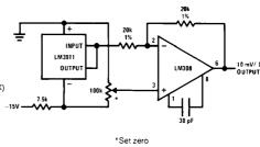
$$R2\left(\Omega\right) = \frac{\left(V_{Z} - 0.01\,T_{L}\right)\left(I_{H} - \frac{0.01\,T_{H}}{R1}\right) + \left(V_{Z} - 0.01\,T_{H}\right)\left(\frac{0.01\,T_{L}}{R1} - I_{L}\right)^{11}}{\frac{0.01}{R1\,R3}\bigg[T_{H}(V_{Z} - 0.01\,T_{L}) - T_{L}(V_{Z} - 0.01\,T_{H})\bigg]}$$
