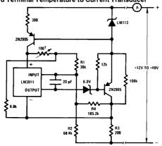
$$R3(\Omega) \ge \frac{V_Z \left(\frac{T_H}{T_L} - 1\right)}{I_H - \frac{I_L T_H}{T_L}}$$
