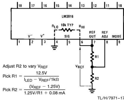
FIGURE 10. Design Equations for Fixed LED Intensity
