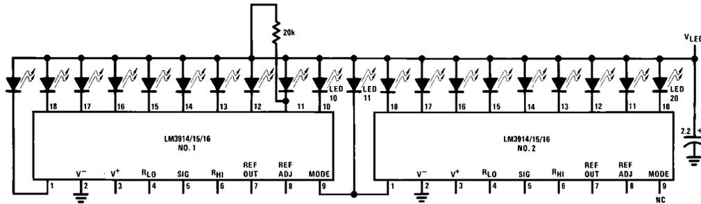
FIGURE 1. Cascading LM3914/15/16 Series in Dot Mode
