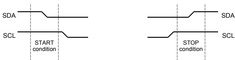
Figure 15-3. START and STOP Conditions
