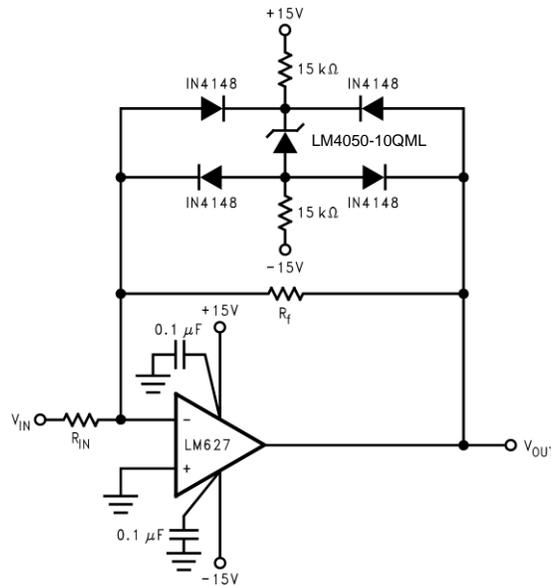
Nominal clamping voltage is ±11.5V (LM4050QML's reverse breakdown voltage +2 diode V<sub>F</sub>). Bounded amplifier reduces saturation-induced delays and can prevent succeeding stage damage.
