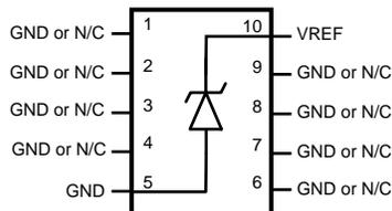
**Figure 1. 10-Lead Ceramic CLGA, Top View**
