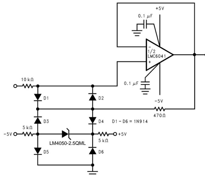
The bounding voltage is ±4V with the LM4050-2.5QML (LM4050QML's reverse breakdown voltage + 3 diode V<sub>F</sub>).
