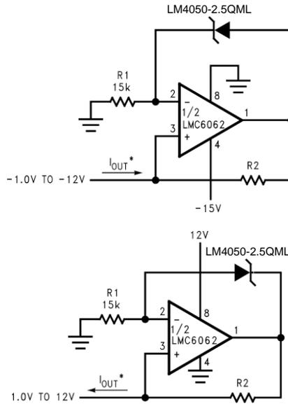
Figure 17. Precision 1  $\mu$ A to 1 mA Current Sources
