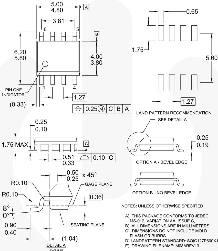
**Figure 19. 8-Lead, SOIC, JEDEC MS 0-12, 0.150 inch Narrow Body**
