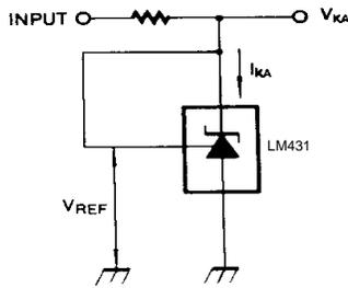
Figure 2. Test Circuit for  $V_{KA} = V_{REF}$
