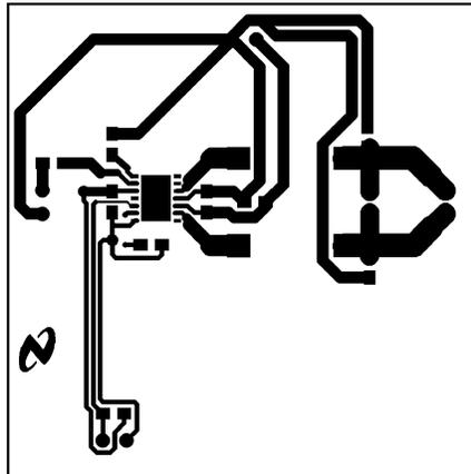
Figure 3. Recommended SD PCB Layout
