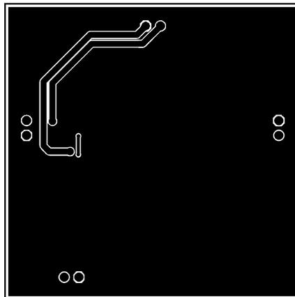
Figure 4. Recommended SD PCB Layout
