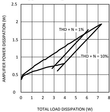
Amplifier Power Dissipation vs Total Load Power Dissipation
