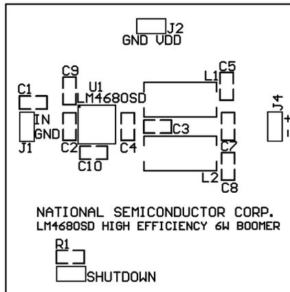
Figure 2. Recommended SD PCB Layout
