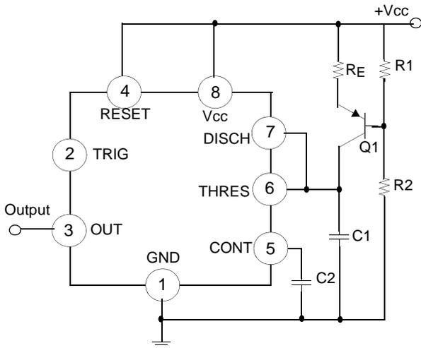
Figure 13. Circuit for Linear Ramp
