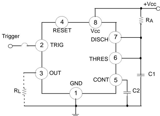
**Figure 1. Monostable Circuit**
