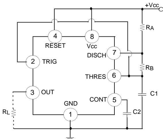
Figure 5. Astable Circuit
