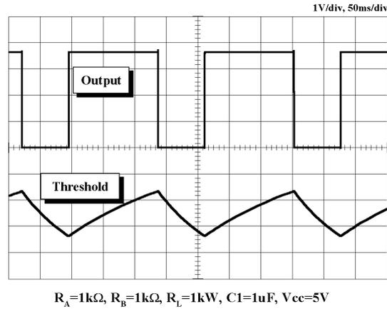
**Figure 7. Waveforms of Astable Operation**
