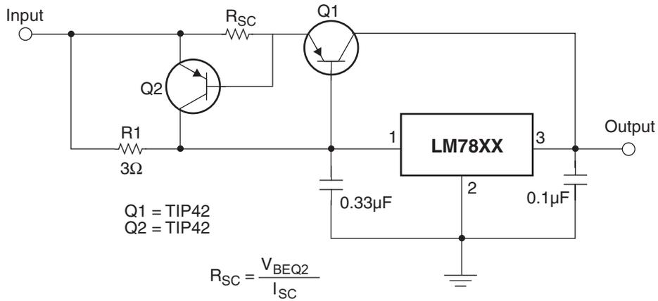
**Figure 15. High Output Current with Short Circuit Protection**
