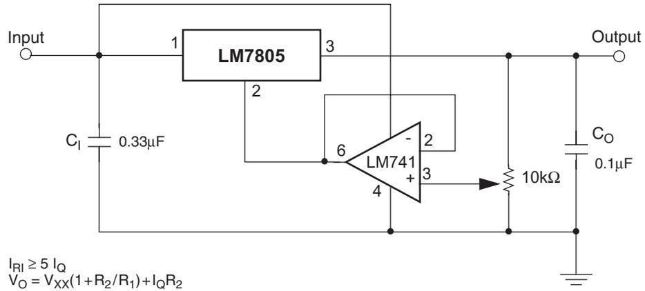
**Figure 13. Adjustable Output Regulator (7V to 30V)**
