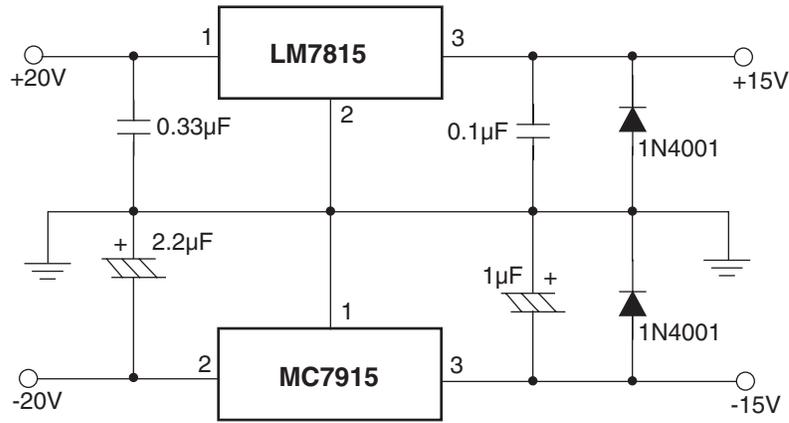
Figure 17. Split Power Supply ( $\pm 15V - 1A$ )
