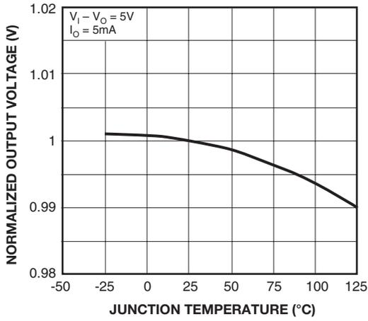
Figure 5. Output Voltage
