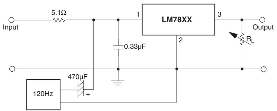
**Figure 9. Ripple Rejection**
