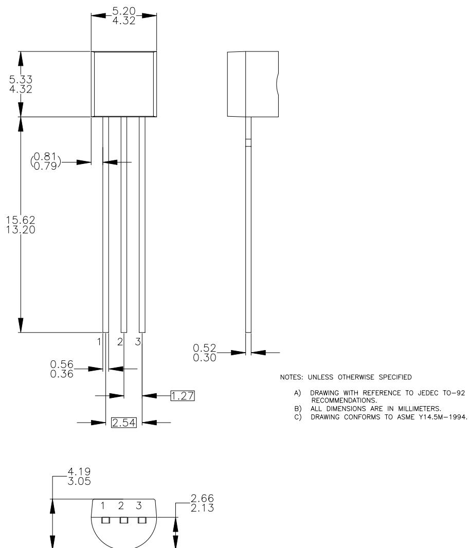
**Mechanical Dimensions** (Continued)**Package****Dimensions in millimeters****TO-92 Formed Lead For T&R and Ammo Packing**
